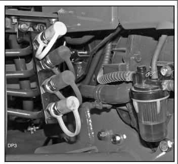
Figure 5. Tractor Hydraulic Couplers
